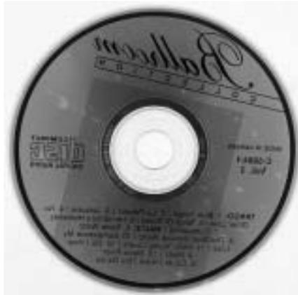
Fig. 3: An audio CD (viewed through the base side) after 84 days of aging. The metal layer has been attacked and is nearly transparent. The label on the other side of the disc can be easily read.
