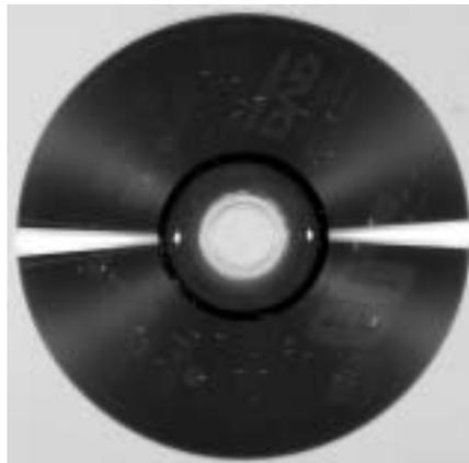
B: Two examples of pinholes in the metal reflective layer.
