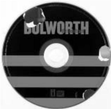
Fig. 2: Audio CD showing small areas of delamination after 84 days of aging. The label, lacquer and metal reflective layers have delaminated in these areas.
