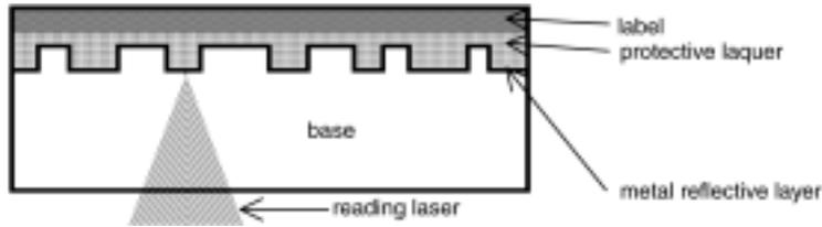
Fig. 1: A cross-section of a read-only or stamped CD such as an audio CD).
