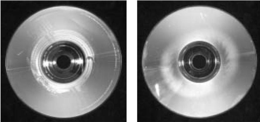
Fig. 6: DVD read-only discs (movie discs) with visible deterioration as a result of accelerated aging. The view of the discs is through the base side.
